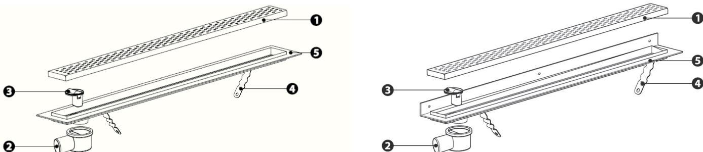
The corner drain is tested for drainage capacity as per ČSN EN 274. If subfloor heating and corner drain are used simultaneously, make sure that the distance of the floor heating is at least 30 cm from the trap - this will avoid undesirable drying.
